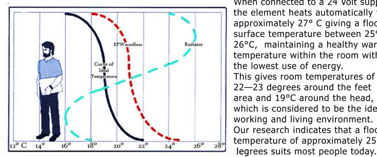
When connected to a 24 Volt supply, the element heats automatically to approximately 27° C giving a floor surface temperature between 25° & 26°C, maintaining a healthy warm temperature within the room with the lowest use of energy. This gives room temperatures of 22—23 degrees around the feet area and 19°C around the head, which is considered to be the ideal working and living environment. Our research indicates that a floor temperature of approximately 25°C
